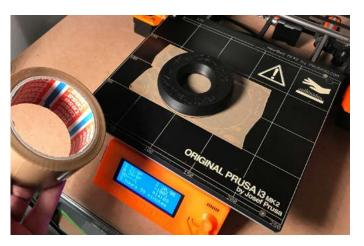
Tip for printing flexible filament (used for printing tyres): it is a good IDEA to use some adhesive tape or foil... first layer adhesion could be too strong or too weak, depending on what filament you use... (picture:RubberJet - TPE32 245/30°C)
