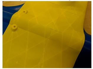
2. Spread CA on the body of each wing nut holder, then drop them into their pockets in the fuselage.
