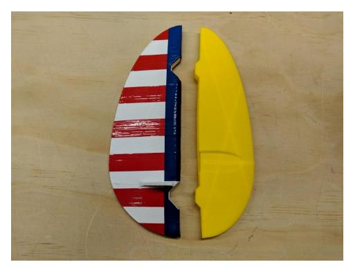
3. Place a drop of glue on each hinge pin, then push them into their mount holes in the vertical tails. Be sure that their rotation axes are aligned with the rudder's hingeline. Then, use activator to secure.
