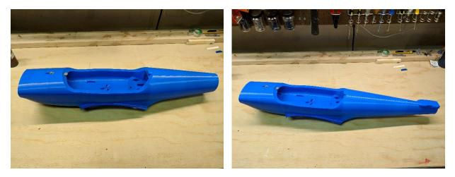
5. Assemble the canopy by joining canopy sections 1, 2, and 3.
