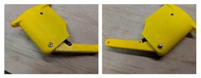
5. Attach the lower end of the shock absorber to the strut with an M2.5 x 10 bolt and an M2.5 lock nut.
