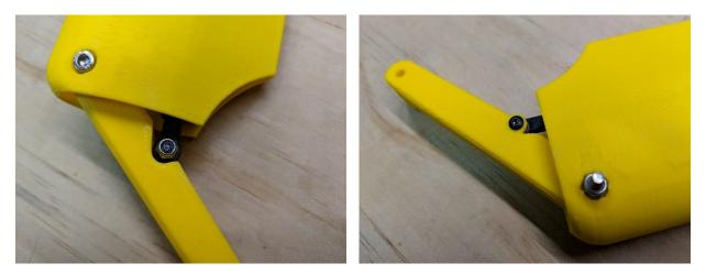
6. Attach the wheel to the strut with an M3 x 40 bolt, three M3 washers, and an M3 lock nut. It should be able to rotate freely.
