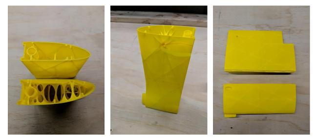
3. Spread glue liberally along the joining faces between the assembled "A" and "B" subassemblies. Join them together, standing the root ends on a flat surface to help maintain alignment. Use CA activator to secure.
