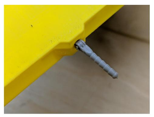
12. Dry-fit the elevator onto the hinge pins and center it, then mark the location of the elevator control horn on the pushrod. Make a z-bend at this location.
