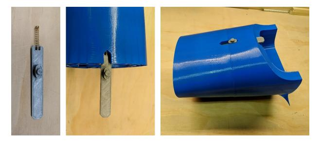
2. Join section 4 to section 3, applying the CA to section 4 to avoid getting glue on parts of the wing saddle that aren't involved in the joint.
