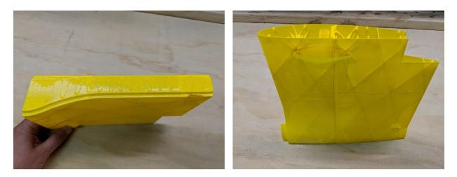
4. Complete the wing panels by gluing sections 3, 4, 5, and 6 in sequential order.
