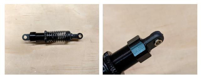
3. Align the top end of the shock absorber (the ball link you just installed) with its mount hole in the gear pylon. Secure with an M2 x 20 bolt and an M2 nut.
