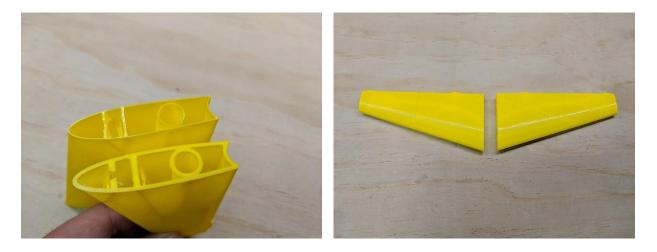
2. Join the rudder sections and vertical tail sections.
