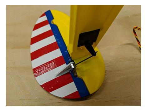
9. Thread the rudder servo leads through the tubes in the fuselage. Glue the completed tail halves onto Fuselage 8, making sure to keep them level.
