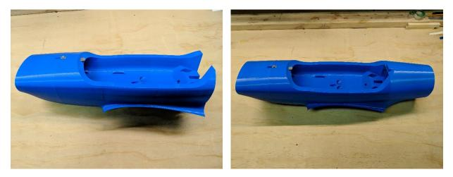
4. Complete the fuselage by joining sections 7 and 8 to the assembly. Do not attach sections 1 or 9 at this time – they'll be joined after the motor and elevator pushrod are installed, respectively.
