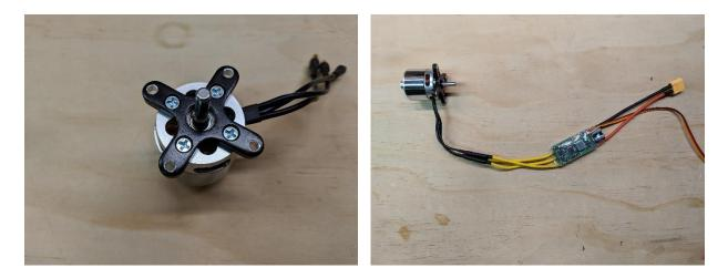
2. Lower the ESC and wiring into the fuselage from the front. Then, use four self-tapping screws to attach the cross mount to the fuselage. You can reinforce with CA for additional strength.
