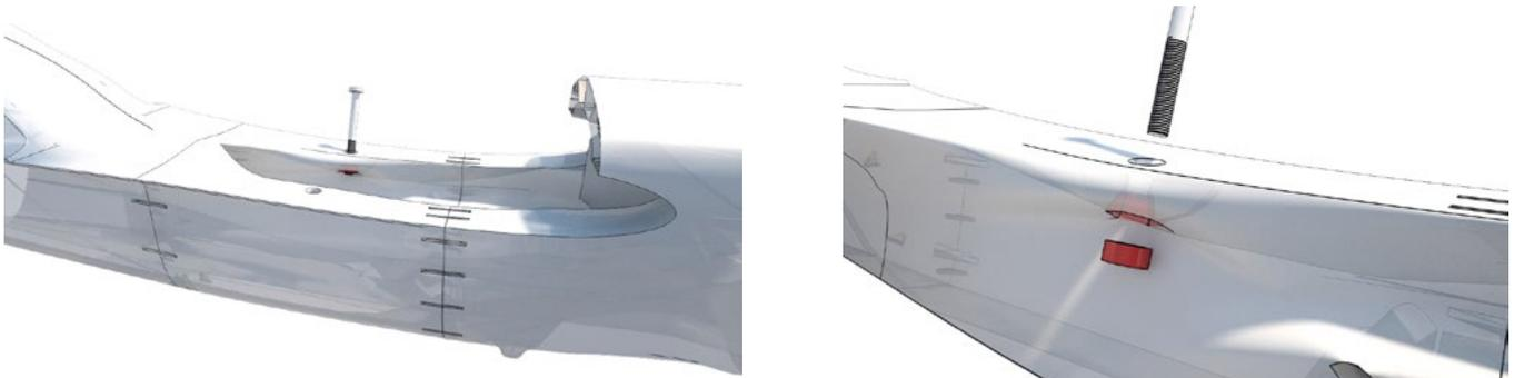
Apply CA glue to the contact surfaces (marked red in the picture) and immediately apply activator as we dont want to CA Glue leak to nuts thread anywhere.
