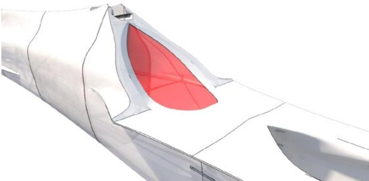
Cut and remove plastic from internal side of fuselage marked in red (use any hot tool).
