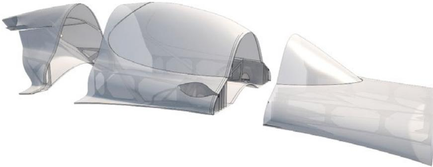
Proceed with fuselage cowling parts 01 and 02, glue it the exactly same way as with previous bayonet coupling wing or fuselage system (alternatively you can use Hannes Arch style cowling):
