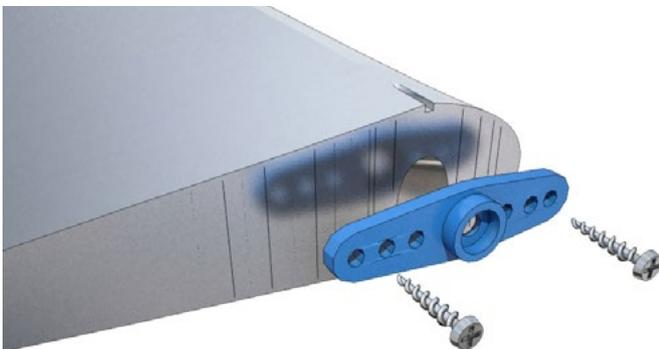
Center servo to its neutral position (user your RC system or servo tester). Attach aileron to axle of servo and again apply Loctite to servo arms bolts, then screw it in properly. **We highly recommend to test the power and function of the ailerons, use your hands to load it, do not worry use abrupt power, it is better if something goes wrong now...:**
