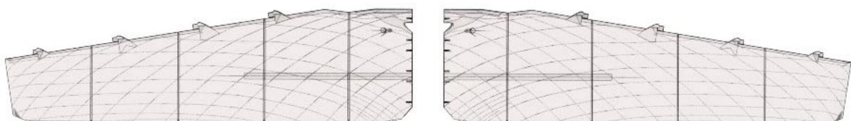
Now you can insert the carbon tube spar... apply CA glue to the contact surfaces (marked red in the picture) and insert carbon tube, press both sides of the wing together, then apply the activator:
