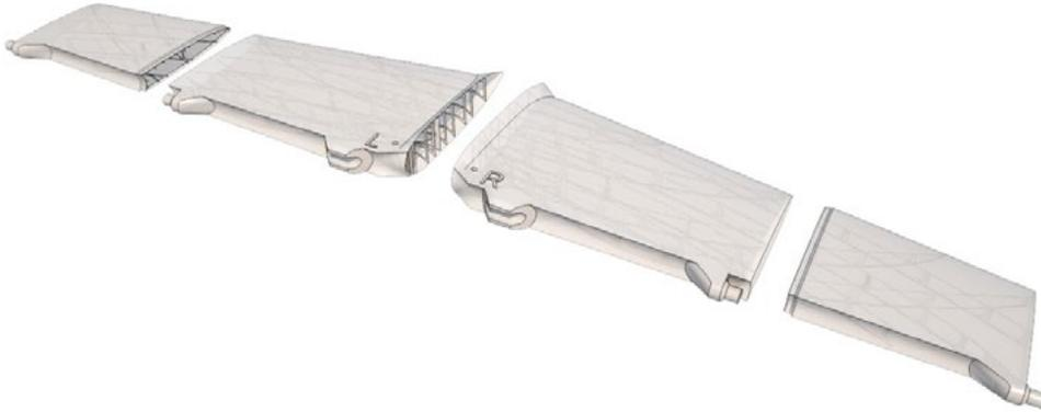
Apply CA glue to the contact surfaces (marked red in the picture) and insert them together, then apply the activator:
