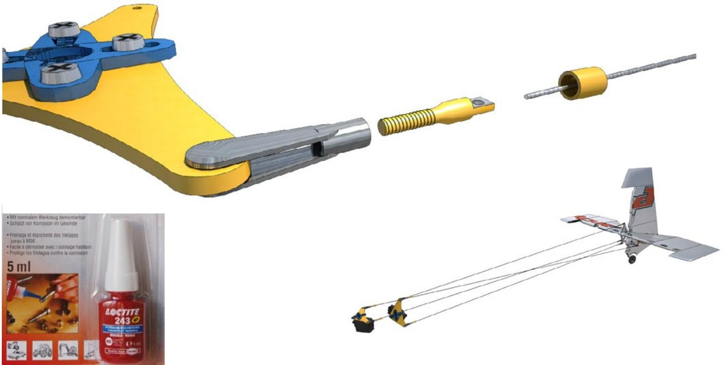
**We highly recommend to test the power and function of the rudder and elevator linkage, use your hands to load both surfaces, do not worry to use abrupt power, it is better if something goes wrong now..., and again use Loctite to both servo arms bolts and all brass ends:**
