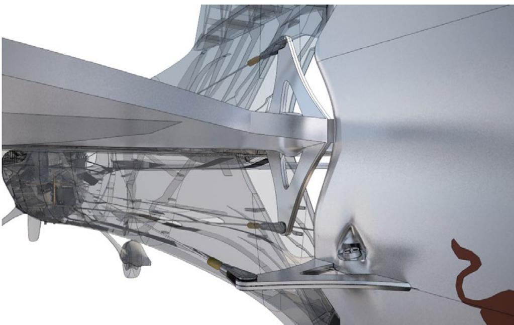
Of course you can use your trusted solution for rudder and elevator pull-pull linkage, we just add some pictures to show you some other options. Always use some thread-locker (Loctite and so on...) and check the function thoroughly on the ground :
