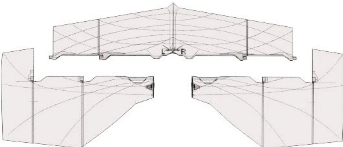
Glue vertical stabilizer to fuselage, apply CA glue to the contact surfaces (marked red in the picture) and insert them together, then apply the activator:
