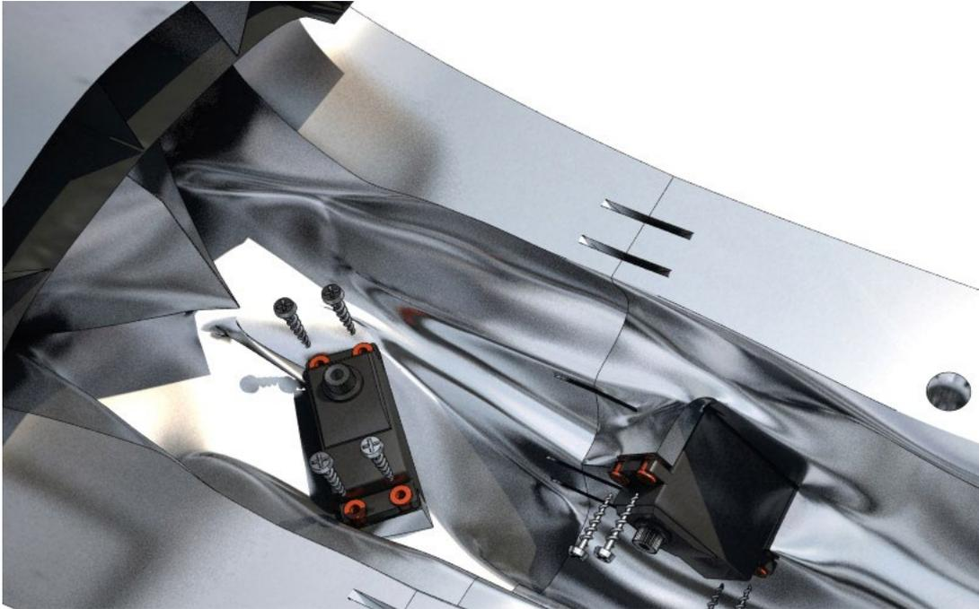
Center servo to its neutral position (use your RC system or servo tester). Put on prepared servo arms, one is suitable for elevator and the other one for rudder (you can find this info on both servo arms):
