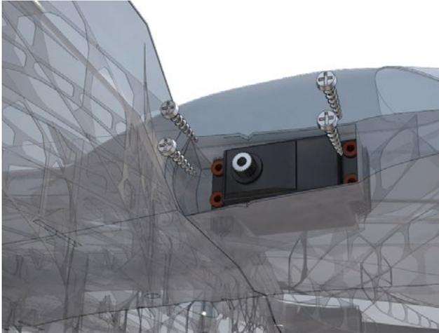
Now attach servos arm to aileron and prepare holes for self-tapping screws with hot 1-1.5mm wire, then screw this screws in. Note: you can use more screws, you know, feeling confident...:
