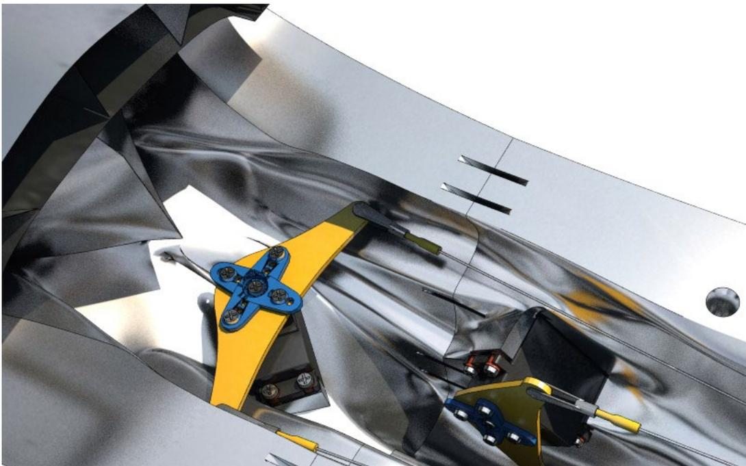
Now finish pull-pull linkage as shown on the picture (servo side), Note: we need light tension in rudder and elevator wires and possibility to tighten up the brass linkage ends in the future. When routing the RUDDER pull-pull wires/linkage through the fuse, they should cross like an "X", but the ELEVATOR should be parallel (as shown on the picture)
