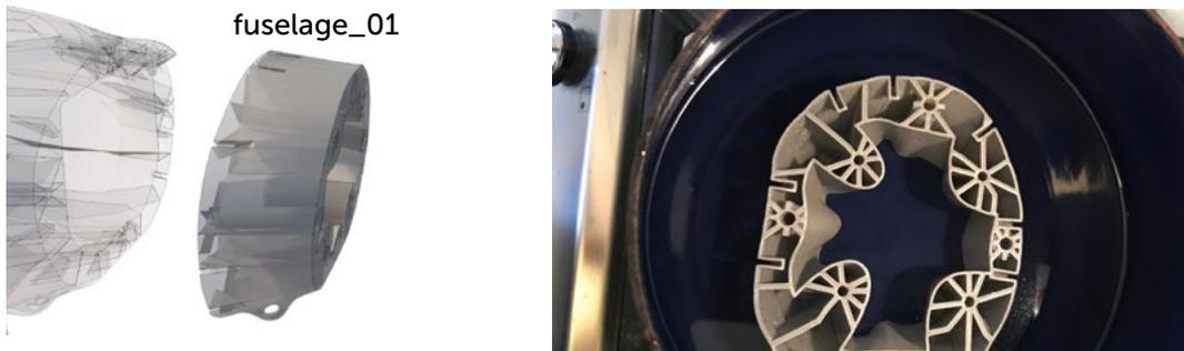
Glue the fuselage parts F1-F9 with CA glue together. You can use snap knife to clear the shape of printed parts, but mostly this is not necessary.
