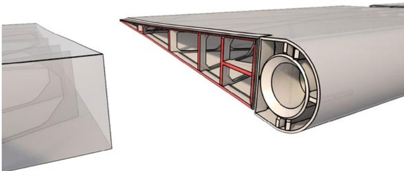
Now you can slide both ailerons to the main wing hinges and apply some oil for better movement:
