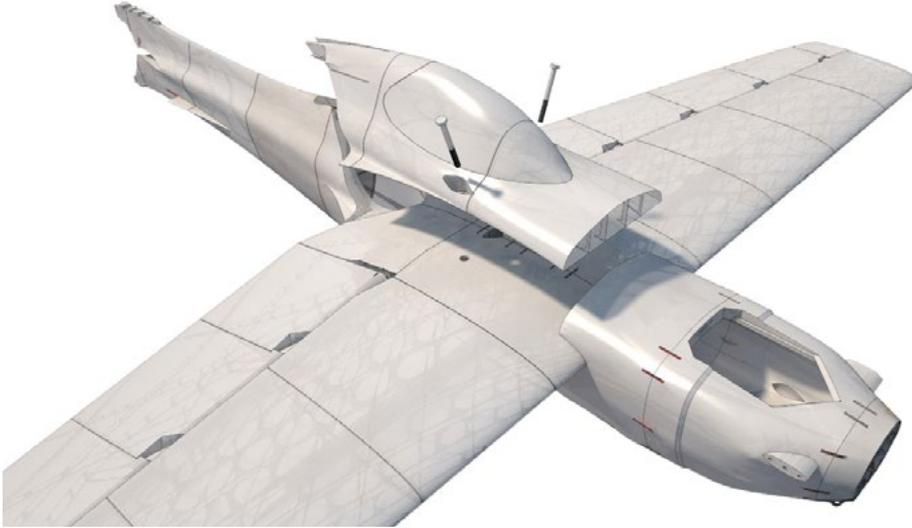
Apply CA glue in the edge between wing and UP fuselage parts **NOTE: don't glue wing with main fuselage:**
