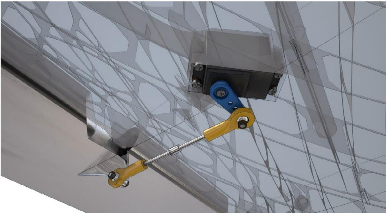
Insert servo into slot, then prepare holes for four self-tapping screws with hot 1-1.5mm wire, you can use any steel wire and any source of fire (firestarter, dremel and so on...) and screw the four screws in. Center servo to its neutral position (user your RC system or servo tester):
