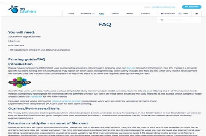
The screenshot shows the FAQ page on the 3D LabPrint website. It includes sections for 'You will need', 'Printing guide/FAQ Introduction', and 'Extrusion multiplier - amount of filament'. The 'Extrusion multiplier' section advises experimenting with the multiplier to achieve the correct weight, noting that a multiplier of 1.0 is often a good starting point.
