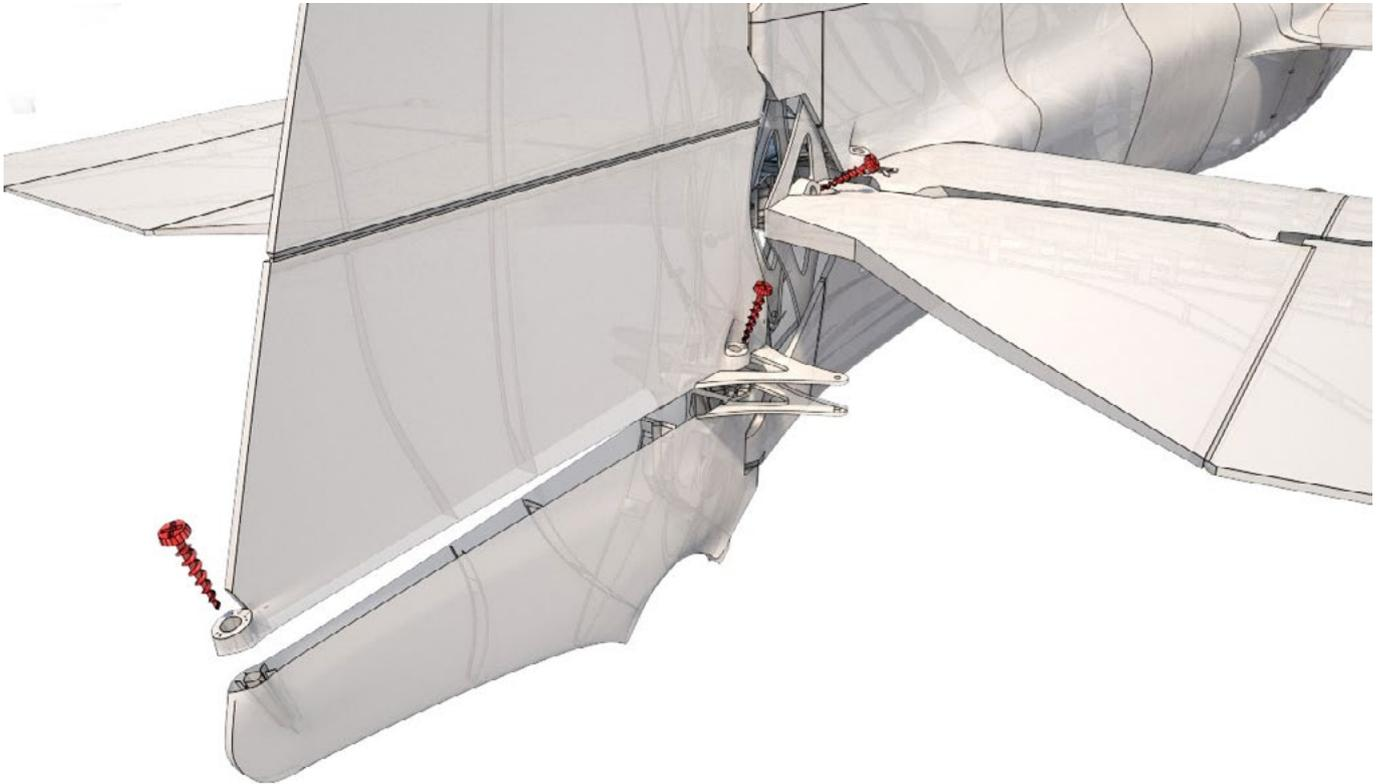
Do not forget the two screws on the bottom side of horizontal stabilizer...:
