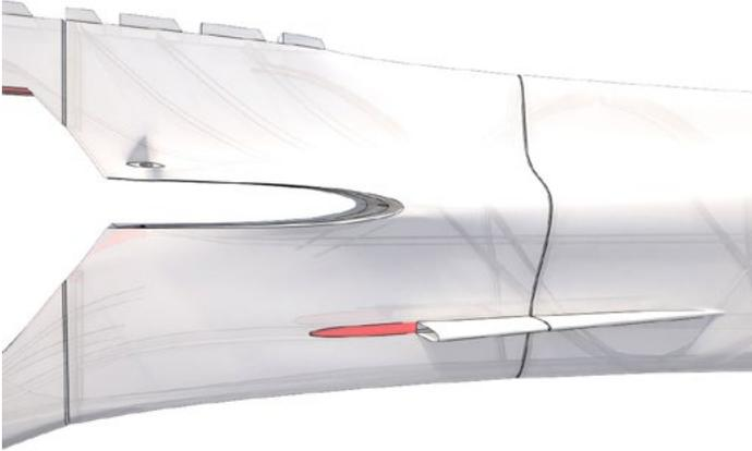
Cut and remove plastic from internal side of fuselage marked in red (use any hot tool).
