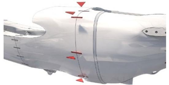
Now you can proceed with next F6 -F9 parts, there is a bit different coupling system (bayonet coupling) procede the way like with wing assembly:
