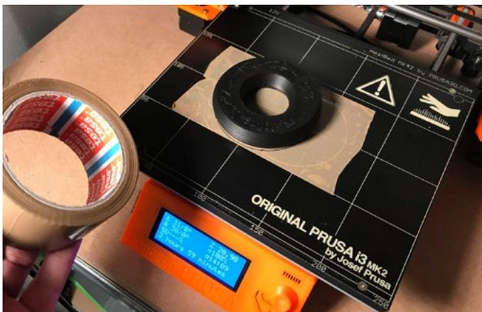
Some advice for rubberlike filament printing (printable tyre): it is a good IDEA to use some adhesive tape or foil... first layer bonding could be too strong or on the other hand too weak depends what filament is used... (picture:RubberJet - TPE32 245/30 print temperature)
