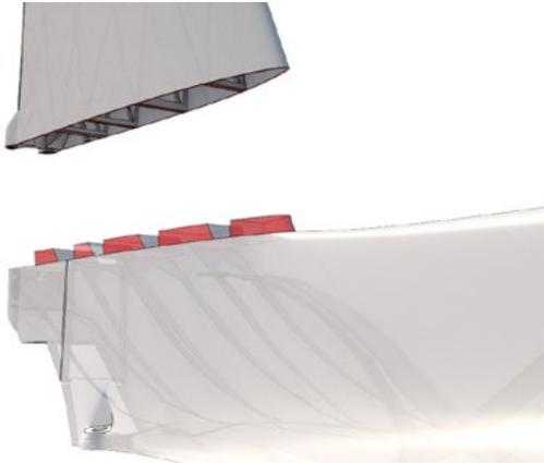
For rudder, proceed the same way like with previous wing parts (RUDDER 2, 3, 4). NOTE: do not glue both Rudder parts together (RUDDER 1):
