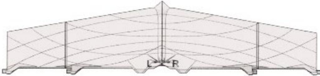
For elevator, proceed the same way like with previous wing parts. NOTE: do not glue both elevators together:
