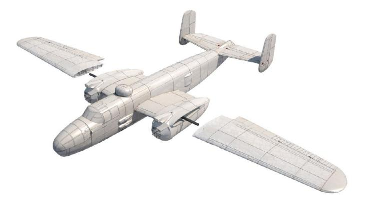
And again, use self-tapping screw to secure the outer wing to the gondola:
