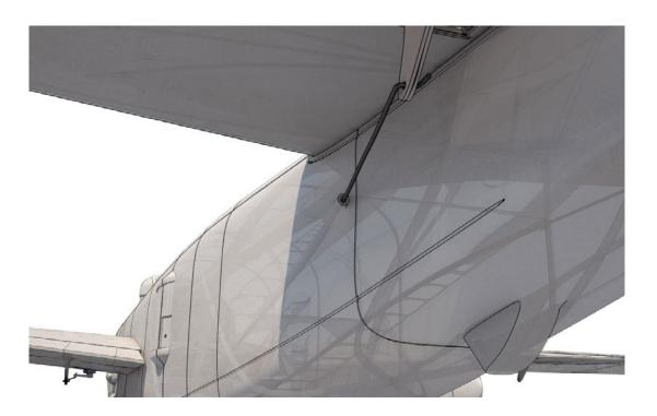
Center servo to its neutral position (use your RC system or servo tester). Attach the prepared servo arms. Remember that you must slide all the servo cables in to the "servo cable tunnel" and the servo cable extension must reach the battery/receiver comparment in the nose of the fuselage.
