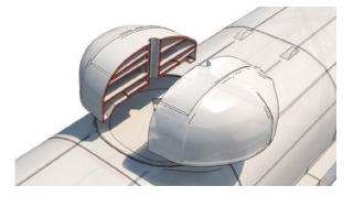
Now battery cover..., cut out both print supports (marked red in the picture):
