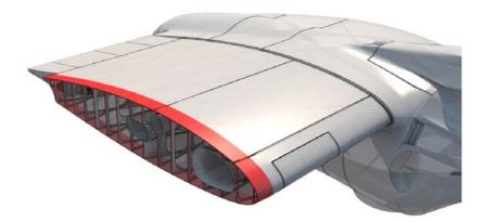
Test fit the parts, then apply CA glue to the contact surface on the wing (marked red in the picture) and insert to the fuselage, finally apply the activator:
