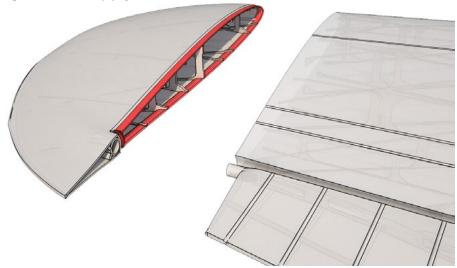
Apply CA glue to the contact surface of the flaps parts (marked red in the picture) :
