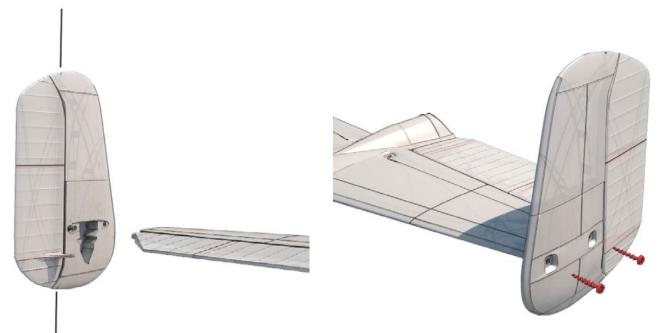
Now you can slide this assembly of tail parts in to the fuselage:
