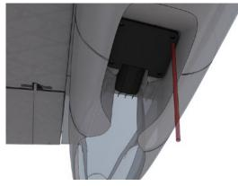
Secure the retract unit using all four self-tapping screws:
