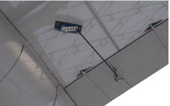
Remember, you must slide all servo cables in to the "servo cable tunnels". The servo cable extension must reach the battery/receiver comparment in the nose of the fuselage.
