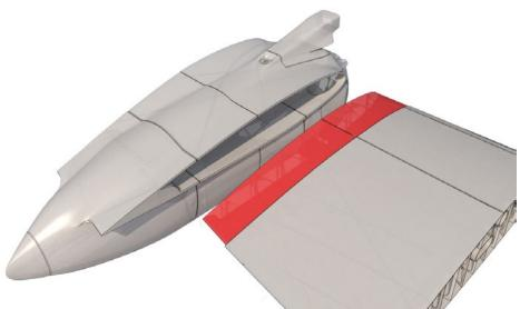
Use any hot tool to cut out the hole (marked red in the picture) for main landing gear wheel:
