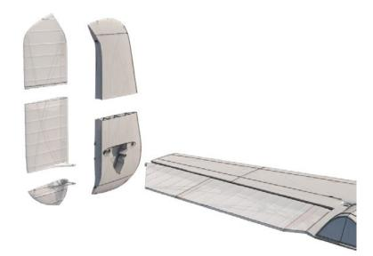
Glue both parts of the vertical stabilizer together (side by side):
