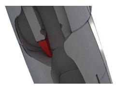
Proceed the same way as with main LG, but here is the difference. Don't remove the 5mm LG pin, but use a shaft coupler to connect the LG leg. Depending on a coupler used, glue it with epoxy or CA glue, tighten the screws or make a solder joint.
