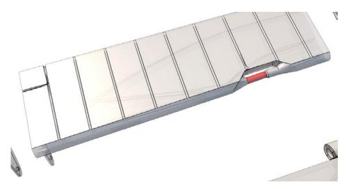
Apply CA glue to the contact surfaces (marked red in the picture) and align the parts together, then apply the activator:
