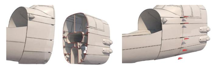
Now you can proceed with next fuselage parts, there is a bit different coupling system (bayonet coupling) proceed the same way as with the wing assembly:
