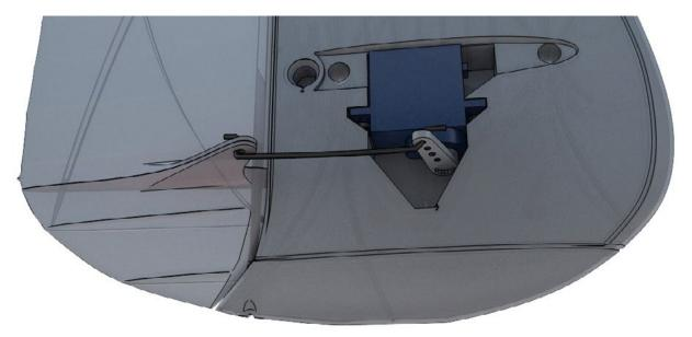
Now mount vertical stabilizer/rudder using two self tapping screws to mount it to the horizontal stabilizer again.
