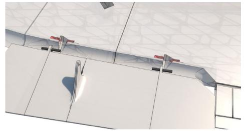
Apply CA glue to the contact surfaces (marked red in the picture) and insert flap with hinge, then apply the activator and operate the flaps till CA glue is completely cured:
