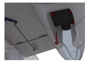
Shape the 5mm steel rod using vice, (you can add fire) and hammer according to the 3D printed template, cut the ends, slide in main wheel and secure it with Wheel Stop Set Colar and threadlocker (Loctite):
