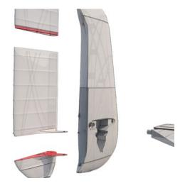
For rudder hinge use a 1.2-1.5 mm wire or carbon rod. Finally use two self tapping screws to mount it to the horizontal stabilizer :
