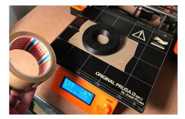
Some advice for rubberlike fillament printing (printable tyre): it is a good IDEA to use some adhesive tape or foil... first layer bonding could be too strong or on the other hand too weak depends what filament is used... (picture:RubberJet - TPE32 245/30 print temperature)
