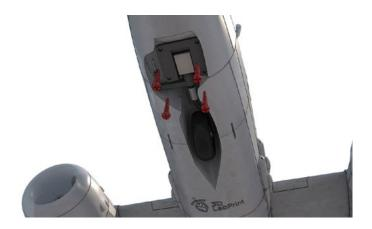
Now add steering servo and linkage, solder the pushrod into the clevis:
