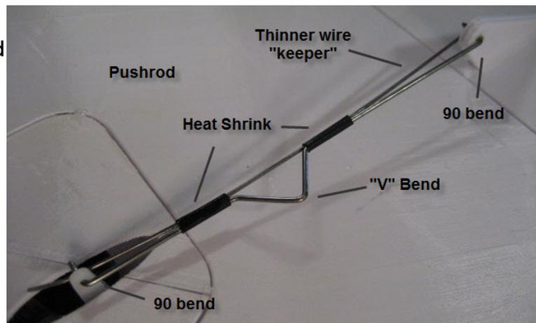
installation and removal. Also notice the extra "V" bend in the pushrod, this is a tried and true method for accurately adjusting the length during the installation.
