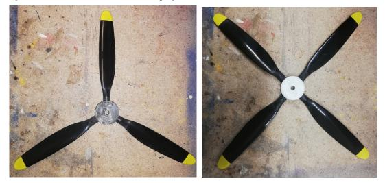
Mount the finished propeller on the motor. Tighten it and make sure that no blade can move inside the hub. <u>As the propeller is exposed to high</u> <u>dynamic radial forces, always work in high quality.</u>
