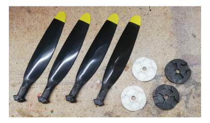
Assembling is pretty easy. Just plug all the blades in one hub part and close the hub with the other half. Don't worry about the gap between the hub parts. It won't cause any problems.
