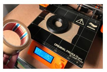
Some advice for rubberlike fillament printing (printable tyre): it is a good IDEA to use some adhesive tape or foil... first layer bonding could be too strong or on the other hand too weak depends what filament is used... (picture:RubberJet - TPE32 245/30 print temperature)
