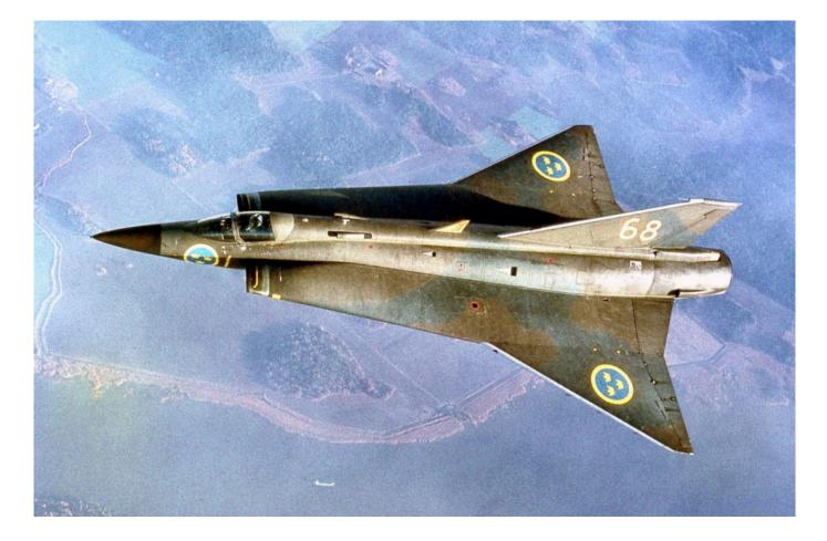
The Saab Draken was developed by Saab in 1955 and was the first fighter aircraft designed with double delta wings. The unconventional wing design also had the side effect of making it the first known aircraft to be capable of and perform the Cobra maneuver. The Draken functioned as an effective supersonic fighter aircraft of the Cold War period. Even though the type was designed and intended as an Interceptor, it was considered to be a very capable dogfighter for the era
