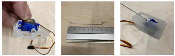
Place the Servos and their mounts in the servo pockets. You can glue the servo mount in place with medium cyano or use 4 small screws to secure each mount. Drill holes with a drill bit of a smaller size than the screws in order for them to get a firm grip. Mount the screws and check the servos are firmly secured.
