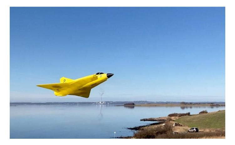
Landings should be performed on a grass strip with short cut grass. Bring the model in low over the end of the grass strip but with enough speed to avoid any stall situation. At very low height over the grass keep dialing in elevator until the model settles on the grass at almost stall speed.
