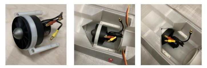
Pull the EDF\_tube out from Fuselage\_07 toward the EDF and route the EDF wires through the hole as shown in the photo. Slide the EDF\_Tube all the way onto the EDF unit. Connect the EDF wires to the ESC. Test the EDF and make sure the sound is "pure whoosh" without any "unwanted" sounds.
