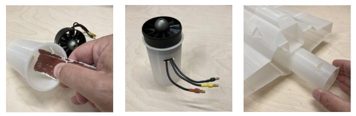
Add Fuselage\_06 to the previously assembled fuselage parts following the same procedure as before. Remember to route the Servo extension wires through Fuselage\_06
