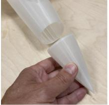
Now it is time to finish the fuselage by adding the final two fuselage parts, Fuselage\_10 and 11. Both parts are printed in the opposite direction of the other 9 fuselage parts. So make sure all edges are nice and clean both on the in- and outside of the parts. Assemble the parts using the same procedure as the previous parts.
