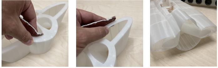
After the hopefully successful assembly of Fuselage\_03 and 04 the two remaining forward fuselage parts Fuselage\_01 and 02 are very easy to assemble. Be aware that Fuselage\_01 has a small mark on the inside flange that indicate the top of the part. You can also look at the location of the stringers which should all line up with the stringers of Fuselage\_02.
