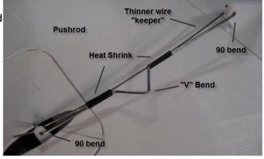
Also notice the extra "V" bend in the pushrod, this is a tried and true method for accurately adjusting the length during the installation.
