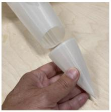
Now it is time to finish the fuselage by adding the final two fuselage parts, Fuselage\_10 and 11. Both parts are printed in the opposite direction of the other 9 fuselage parts. So make sure all edges are nice and clean both on the in- and outside of the parts. Assemble the parts using the same procedure as the previous parts.
