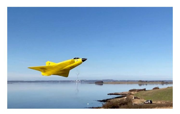
Landings should be performed on a grass strip with short cut grass. Bring the model in low over the end of the grass strip but with enough speed to avoid any stall situation. At very low height over the grass keep dialing in elevator until the model settles on the grass at almost stall speed.
