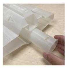
Add Fuselage\_06 to the previously assembled fuselage parts following the same procedure as before. Remember to route the Servo extension wires through Fuselage\_06
