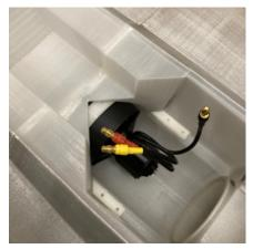
Pull the EDF\_tube out from Fuselage\_07 toward the EDF and route the EDF wires through the hole as shown in the photo. Slide the EDF\_Tube all the way onto the EDF unit. Connect the EDF wires to the ESC. Test the EDF and make sure the sound is "pure whoosh" without any "unwanted" sounds.
