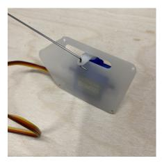
Place the Servos and their mounts in the servo pockets. You can glue the servo mount in place with medium cyano or use 4 small screws to secure each mount. Drill holes with a drill bit of a smaller size than the screws in order for them to get a firm grip. Mount the screws and check the servos are firmly secured.
