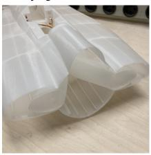
After the hopefully successful assembly of Fuselage\_03 and 04 the two remaining forward fuselage parts Fuselage\_01 and 02 are very easy to assemble. Be aware that Fuselage\_01 has a small mark on the inside flange that indicate the top of the part. You can also look at the location of the stringers which should all line up with the stringers of Fuselage\_02.
