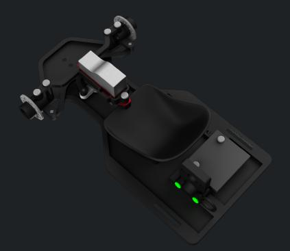
Secure N20 motor with M1.6×4mm screws.
