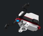
Secure steering links and servo horn with M1.6×4mm screws. Two arms of steering links has to move freely but without any wobble. Use grease for more smooth movement.
