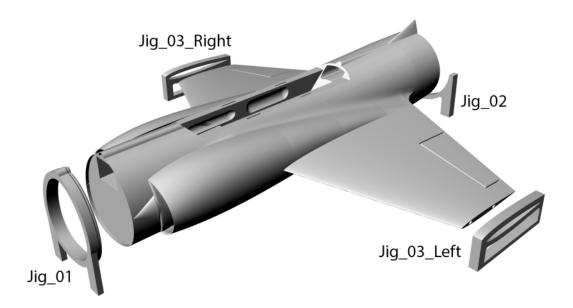
Start with the left wing. Glue two Wing Joiners into the wingroot. You can use a wing joiner to clean out the stringing in the slots as shown in the photo. Press Jig\_03\_Left onto the wingtip. Repeat the process with the right wing.
