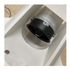
Place the EDF in its correct position and fix it with two servo screws. Make sure the wires from the EDF enters the hole in a nice way by pulling the ESC out of Fuselage\_07 until the wires are taut. Also make sure that the exhaust duct can be fitted on the EDF.
