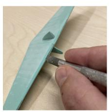
Cut four 6x15mm hinges from cyano hinge sheet. Glue the hinges into the hinge pockets of the horizontal stabilizer. Do not mount the elevator yet. Make a elevator pushrod from 1mm piano wire with a length of 135mm and with z-bends like shown in the photo below. Wrap a standard 3.7g servo with painters tape.
