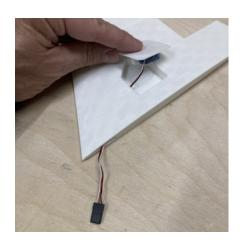
Insert the hinges and mount the aileron. When satisfied with the fit put a drop of thin cyano onto the hinges right at the hinge line. Wipe excess cyano of with a toothpick or similar. Be careful not to get cyano between the aileron and the trailing edge. The aileron should move freely up and down.
