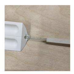
Insert the latch and spring into the slot in Hatch\_01. Press the latch all the way in and test the action of the latch. Pull the latch out again and add glue into the recess on the latch. Use medium cyano and be careful not to get glue between the hatch and the latch. Push Canopy\_Lock\_02 through the slot in the hatch and into the recess. Spray with accelerator. You should now be able to operate the latch mechanism by moving Canopy\_Lock\_02 back and forth.
