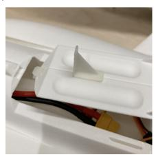
The Starfighter is designed to be launched with a catapult/Bungee launcher. Glue the bungee hook into the recess in Fuselage\_04
