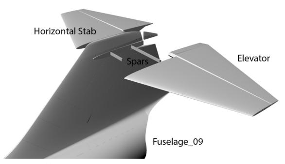
Remove stringing from the spar holes in the horizontal stabilizers. Use a small screw driver or similar to clean the holes. Push the Horizontal\_Stab\_Front\_Spar and Horizontal\_Stab\_Front\_Rear into the holes. Push the two stabilizers together. They should be able to be pushed almost completely together. If not, then try to clean the holes some more. If the stabilizers still can't be pushed together, you can cut the spars to make them shorter.
