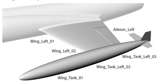
Start by gluing Wing\_Left\_01 and Wing\_Left\_02 together while pressing the parts down onto a flat surface. Cut 8x15mm hinges from cyano hinge sheet. Alternatively you can cut hinges from blister packaging. Just make sure to sand the surface matt with semi coarse sanding paper. Use an exacto knife to open the hinge pockets of both the aileron and wing.
