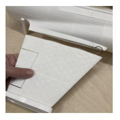
Feed the wires into the fuselage while mounting the wings and make sure the wing joiners are inserted correctly. Place the center section and the jigs on a flat surface. Check that the wings are seated correctly and the base surface of the jigs are touching the flat surface as shown in the photos.
