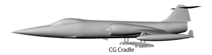
Before first flight make sure the model balances at the Center of Gravity, CG which is indicated underneath the wings by two recesses.
