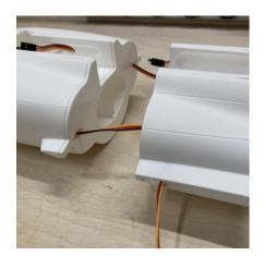
Now it is time to prepare Fuselage\_07 for the 50 EDF unit. Start by routing a servo extension wire through the part as shown in the photos.
