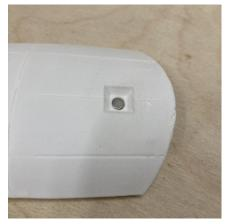
Glue Ventral\_Fin\_Left and Ventral\_Fin\_Right together. Glue a magnet into the recess of Fuselage\_08
