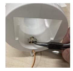
Trial fit the EDF. The XFly Galaxy EDF has flanges for mounting. Mark the position of the flange holes with a felt pen. Remove the EDF and drill pilot holes for two servo screws. You can make a drill by cutting a length of 1mm piano wire and mount it in a power drill. Remove the tape from the ESC wires and connect them to the EDF. Test that the EDF is blowing air in the correct direction.
