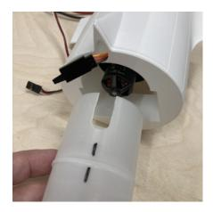
Pull the ESC through the hole in Fuselage\_06 and glue Fuselage\_07 to Fuselage\_06 as shown in the photos.
