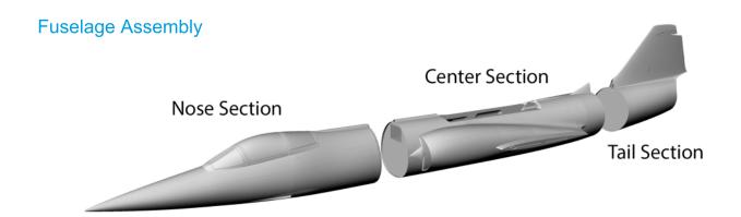
The Starfighter should be built in three separate section: nose section, center section and tail section.
