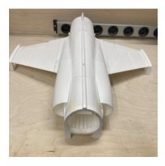
Remove the jigs. The center section is now finished and can be joined with the front section.
