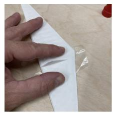
Glue the Vertical\_Fin\_Extension onto the elevator. There is a mark on the elevator indicating the correct location of the Vertical\_Fin\_Extension. Use an exacto knife to open the hinge pockets of both the elevator and the horizontal stabilizer.
