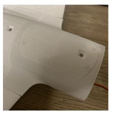
Protect the fuselage with thin plastic film and place two magnets on top of the two magnet in the recesses. Add medium thick cyano glue to the magnet holes of the ventral fin and place it on the fuselage. Make sure the ventral fin is pointing straight down when model is in flying straight.
