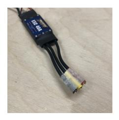
It may be necessary to cut the opening with a pair of scissors as shown. Push the ESC and its wires into Fuselage\_07 until the wires reach the opening. Use a Needle nose pliers or similar to pull the three wires out as shown in the photo.
