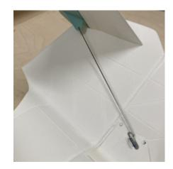
The three sections can now be joined. Glue the nose section to the center section. Connect the elevator servo wire to the servo wire extension from the center section. Pull the elevator servo wire into the center section and glue the tail section to the center section.
