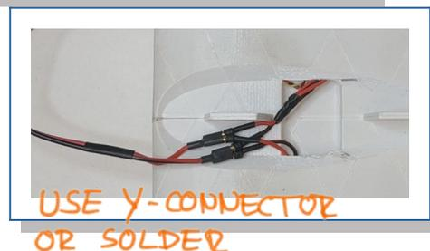
**Hint:** It figured out, that permanently connecting the ESCs isn't very handy. So I recommend creating a Y-connector cable instead. Solder AWG cables to a XT battery-connector, then use the same pins and plugs as from the ESC to motor to create the Y-connection.
