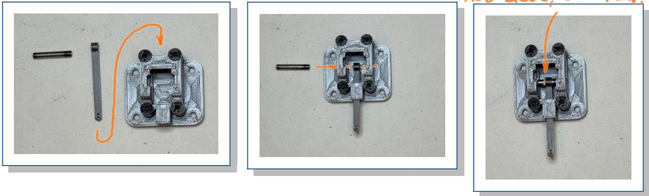
16. Now insert the steer axle into the central piece and both into the base. Use two m3x6 pan head screws to join, tighten carefully and check travel again.
