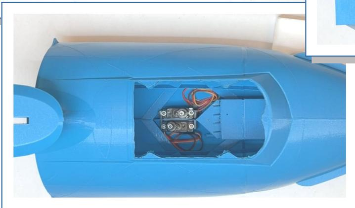
7. Glue together the left and right axle-supports, line up with the other parts according to drawing and hook the door and servo push-rods to the control horns.
