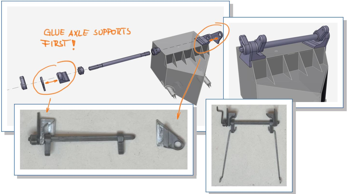
8. Cut the openings for the door push-rods, ad a tiny drop of CA to the free axle support and glue it to the right rear corner of the nose-gear bay. Guide in the door push-rods and fit the axle into the support. Check for alignment, and glue in the other support. the unit to position on the nose-gear bay. Check for correct alignment and add a little accelerator to cure.
