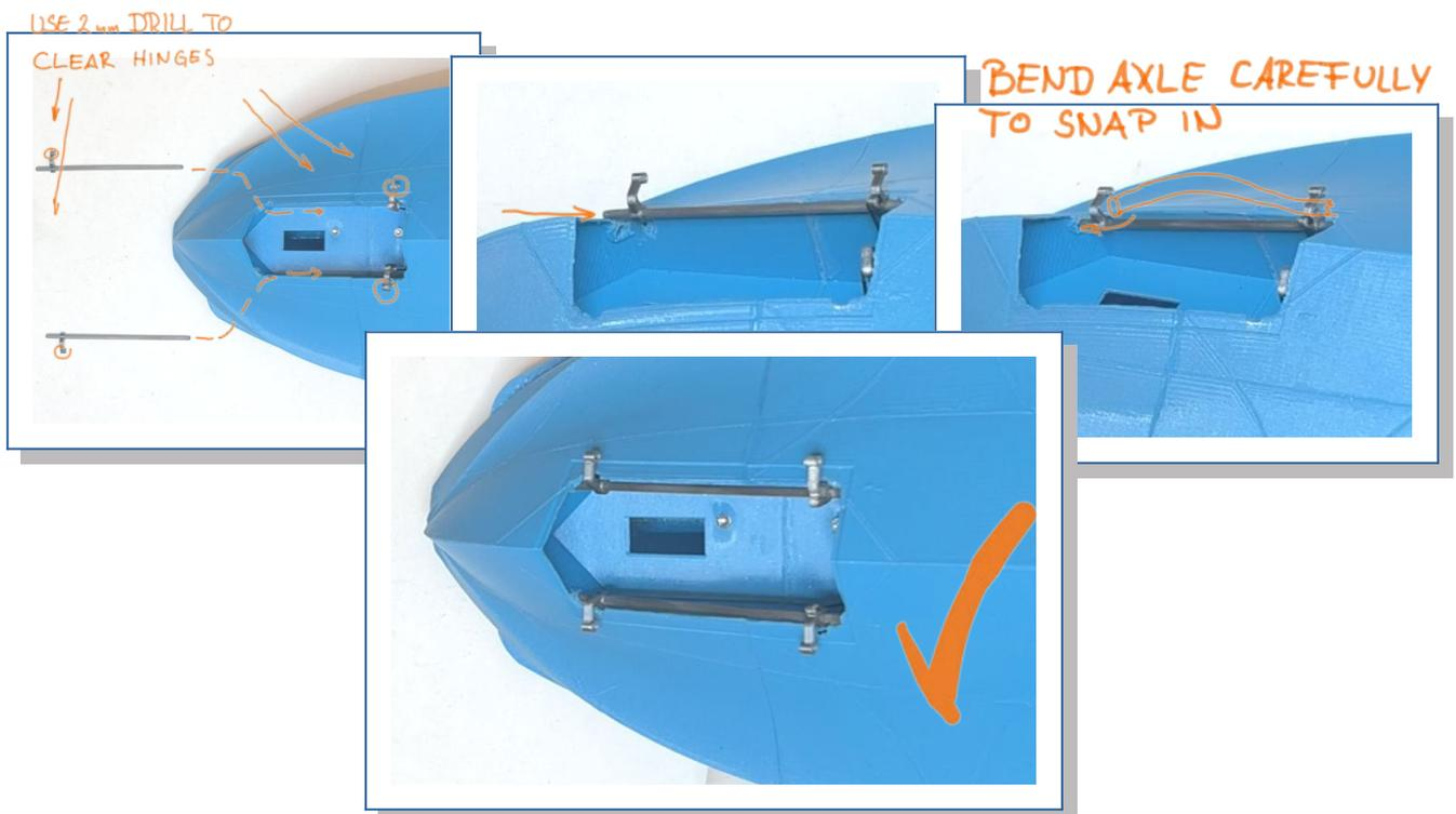
11. Take the gear doors and apply two m2x7 cylinder screws each, but set in only a few turns to keep clear the opening for the hinges. With the hinges in "open" position bring in first door and use a long Allen key to close the screws. Move door and adjust cut-out if necessary, continue with second door.
