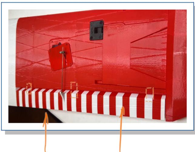
4. Insert the cable-loom into the pylon and place the wing onto the fuselage. Then secure with the m5 nylon screws and nuts and cut the rear screw to length.
