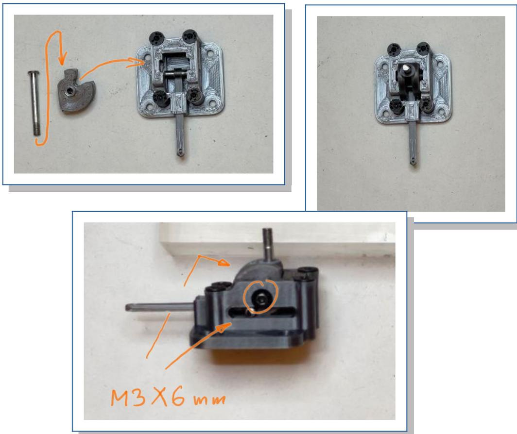
17. Create the nose-gear sliding rod according to wire sheet, pick up the steering lash and insert into the control horn of the front fork from top, secure with CA. Turn in a m3x6 cylinder screw, but don't tighten yet.
