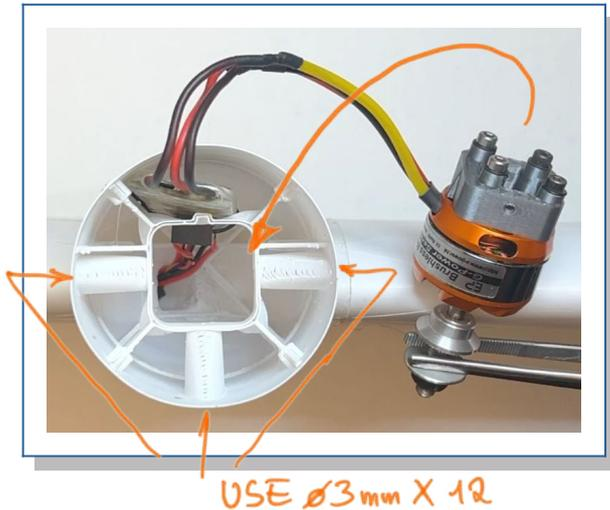
6. Finally use zip ties to arrange the cables in the wing centre, and create a nice cable loom.
