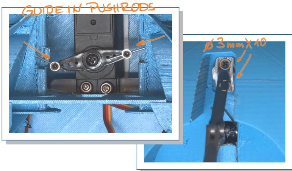
10. Fix the upper and lower arms to the fuselage ( $\varnothing 3\text{mm} \times 10$  self tapping) and then connect to the bumpers using  $\text{m}3 \times 8$ ,  $\text{m}3 \times 10$  and  $\text{m}3 \times 16$  screws. With the servo horn still in horizontal position unfold both sides of the gear by hand, then lock the push rods with the set screws. Use a servo tester or your RC to check for any collision and remove in case.
