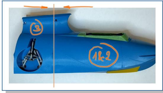
2. Use hot-tool to cut a 10mm x 10mm opening into the bulkhead of #3 for the servo cables.
