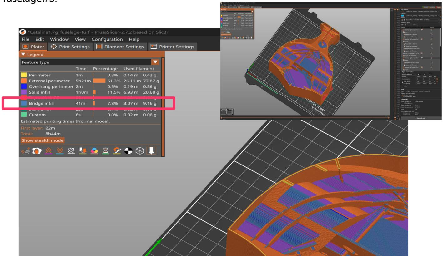
The light blue lines, called bridge infill, appear when you turn on top and/or bottom layer in the print-settings. PS uses these as "quick and cheap" supports for unsupported overhanging top or bottom layers, which might cause the print to fail.
