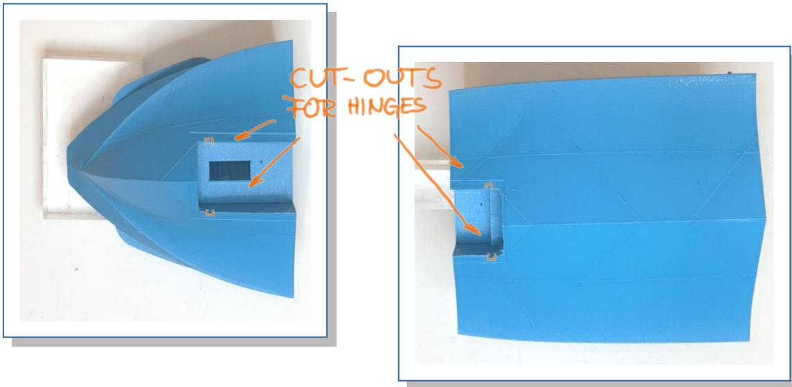
2. Use a long 3mm drill or a round file to carefully clean the door-axle bushings in the fuselage sections #1 and #2 and fit in the door axles. As the axles tend to have a tiny bulge from printing at the tips, start with sanding a little chamfer there and then sand or draw the top and bottom areas, repeatedly checking for fit and depth in the bushings of the fuselage. The axles should turn smooth, without sound and clamping and dive in about 8mm to the front bushings and 10mm into rear ones.
