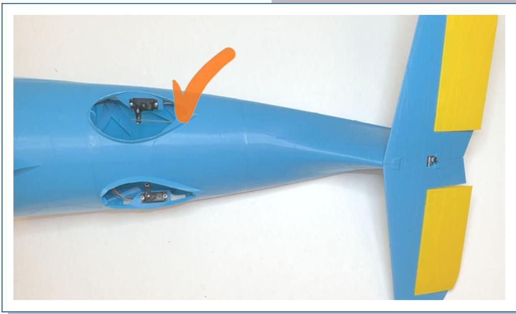
10. Glue the fin onto the elevator, then the two ruder parts together, followed by attaching the hinge into the fin.
