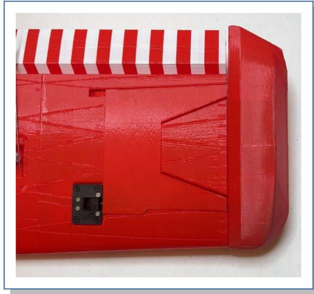
3. Glue together the ailerons and install CA-hinges to. Then Z-bend and cut the aileron-rods according to wire-pattern, link to aileron-horns. Slide hinges into wing and use CA to fix.
