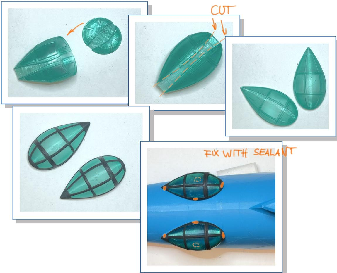
13. Join (and paint) the front canopy, then glue five  $\varnothing 5 \times 1$ mm neodymium magnets to the mount points in the fuselage and stick m3 or m4 washers as counter-pole to the front canopy. (If flying in the water I recommend to pierce holes and using servo screws instead of the magnets.)
