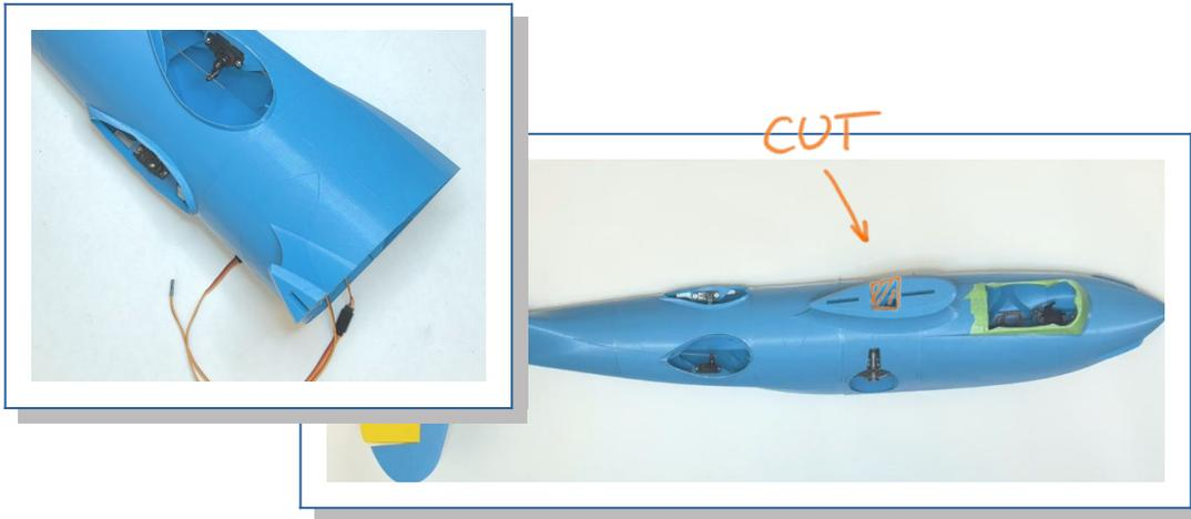
12. Join the rear canopy parts using CA, then divide the "egg" with the hot-tool and clean the edges. Add some colour to the frame, if wanted and use tiny dots of sealant to fix the bulbs to the fuselage.
