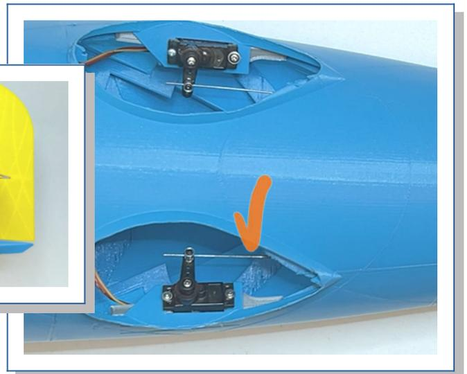
11. Apply extension cables to the servos and guide the plugs through the opening of the bulkhead, then glue together front and rear part and finally cut an opening for the wing-cables into the pylon.
