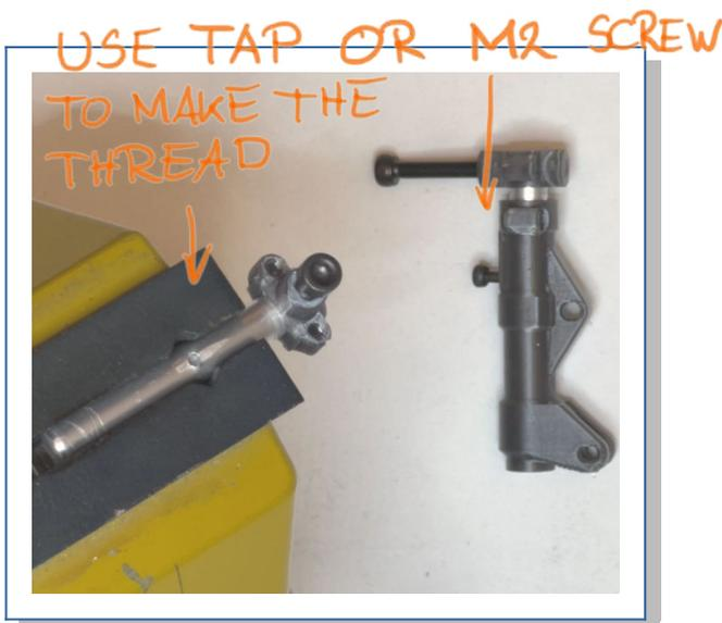
*Hints: 1. Use file and make a small plane, where you plan to puncture and drill.
