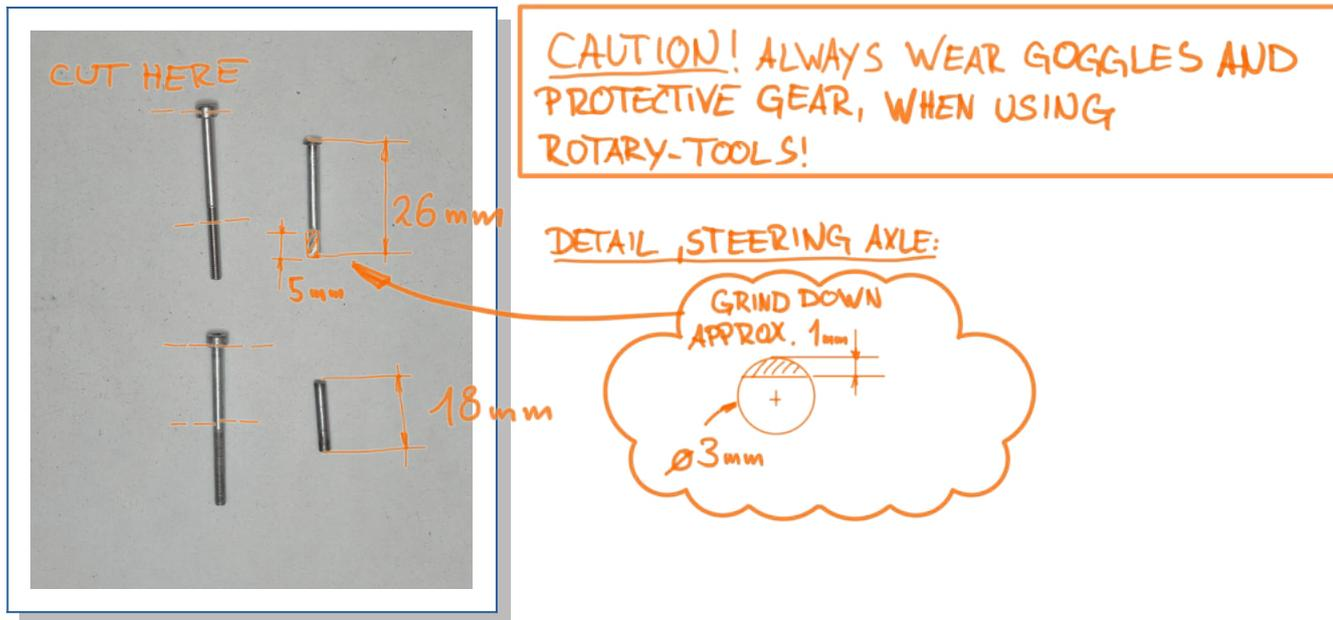
14. Take the nose-gear base and fit with one m3x12, one m3x14 and two m3x16 countersunk screws.
