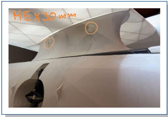
5. Now take the m2x7 cylinder screws and install the wing struts. (Install the longer ones to the front.)
