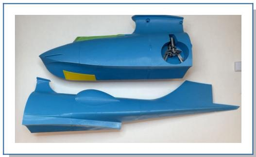
4. Use hot-tool to open the blisters. Leave about 5mm brim on the fuselage.
