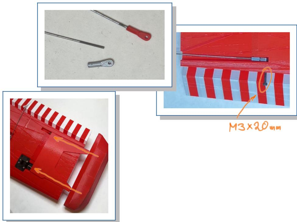
2. Glue together the floater, mind for left and right part and bring some glue into the holes, then slide on the support-rods. Align wing-cover with its cut-out in the wing and use accelerator to fix floater. Repeat with other side.
