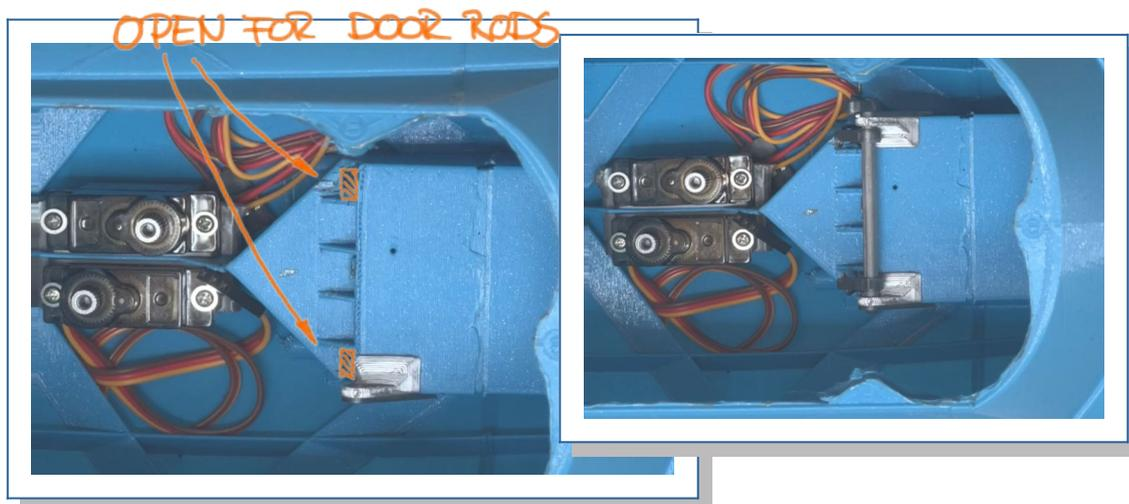
9. Fix another MG90S servo to the last servo-mount, add a short servo horn and hook the unit to the short door pushrod. Fix with two  $\varnothing 3 \times 10$ mm self tapping screws from inside the nose-gear bay.
