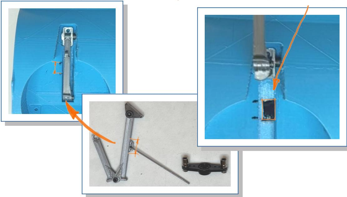
9. Install the servo horn and bring into horizontal position, then guide the push rod into the connector and mount the strut with two  $\varnothing 3\text{mm} \times 10$  self tapping screws.
