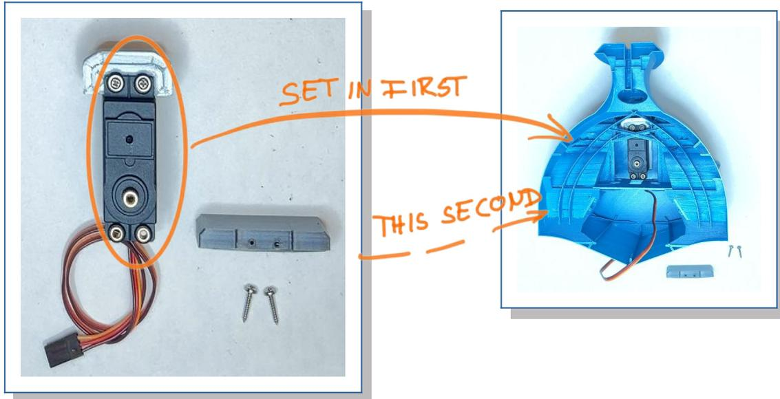
2. If necessary cut an opening into the bulkhead. Then bring the lower servo-mount into position and attach it to the servo as well, check if the servo is aligned correctly with the bulkhead and glue the mounts to the fuselage.
