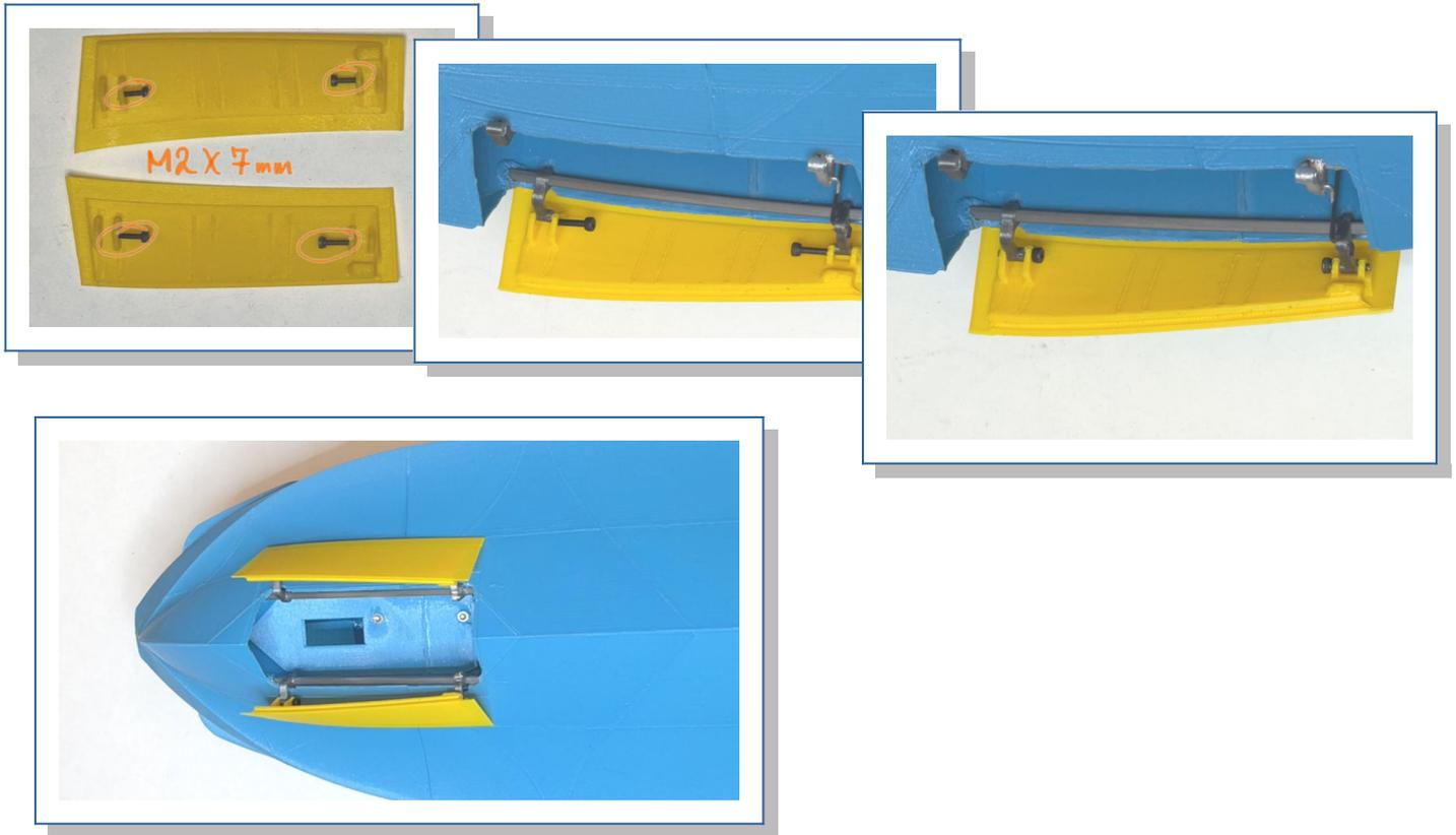
12. Clean the chamfered holes of the two guiding levers and check if screws settle well in, then use long Allen key and m2x6 countersunk screws to connect the levers to the pivot points in the bay. Tighten only lightly! Swing levers to the outside and use m2x10 countersunk screws to connect to the gear door, also close lightly, then check for ease of movement.
