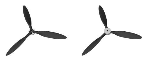
Mount the finished propeller on the motor. I recommend to secure the nut with bolt adhesive or use a self securing nut. Tighten the propeller and make sure that no blade can move inside the hub. <u>As a propeller is exposed to high dynamic radial forces, always work in high quality.</u>
