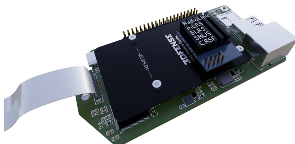
Fully assembled stack with passive cooler and RadioLink module (mLRS / ELRS / SBUS / CRSF)
