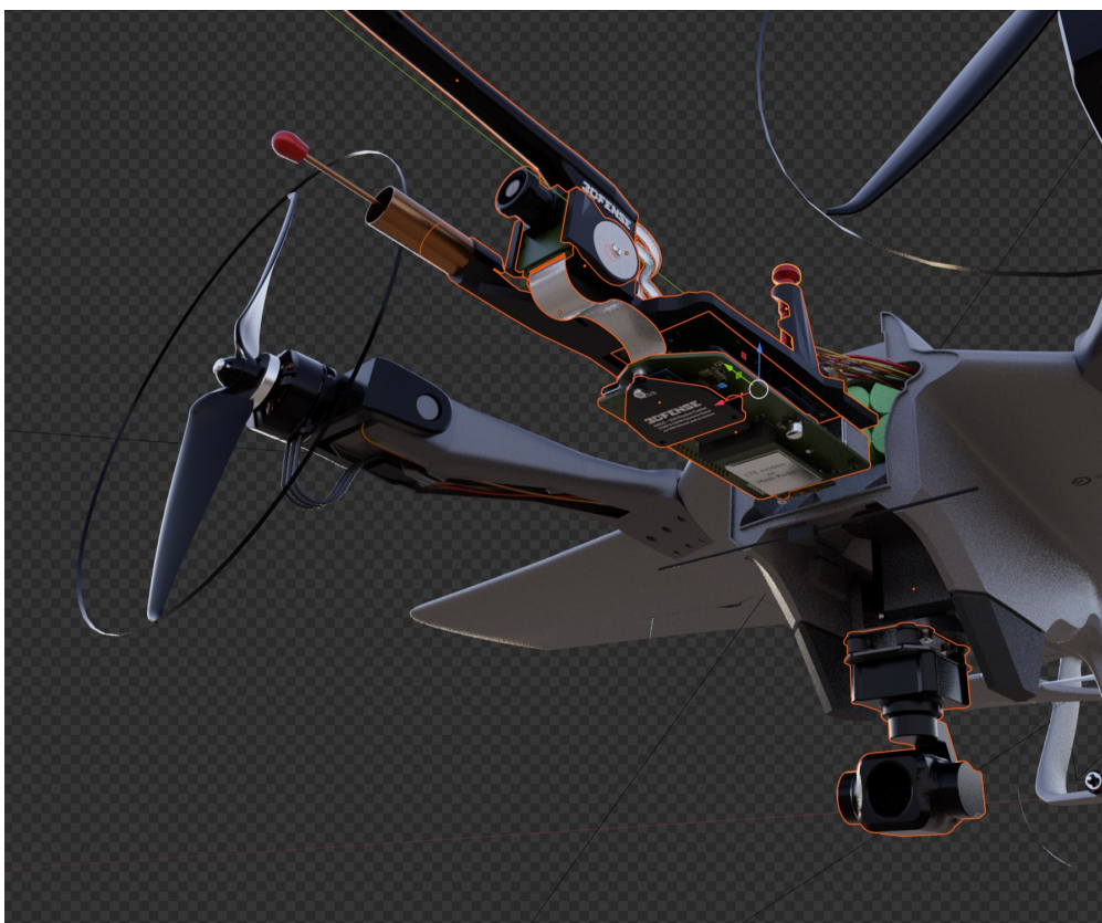
The whole stack in its element — NavPack + CM5 module on the slide-out avionics tray of the D-22 Twin Iron, gimbal camera below (design view)
