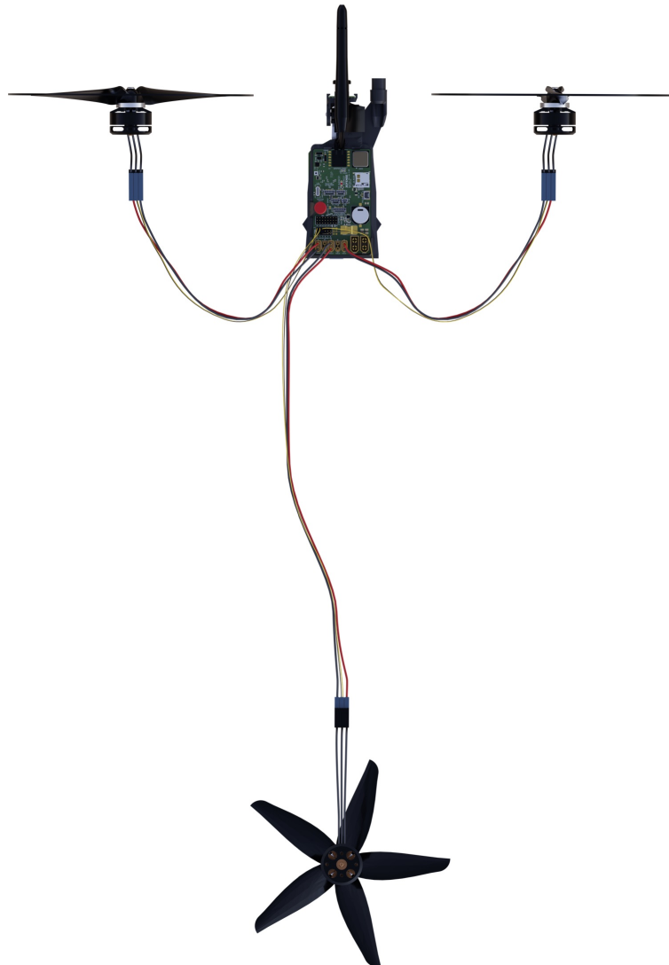
Example propulsion wiring — lift motors and cruise motor, ESCs powered directly from the XT30 outputs
